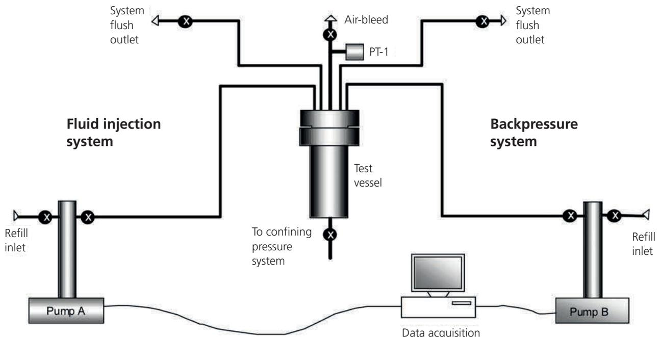
Figure 4.4: Schematic configuration of the BGS permeameter after Harrington et al. (2001).
