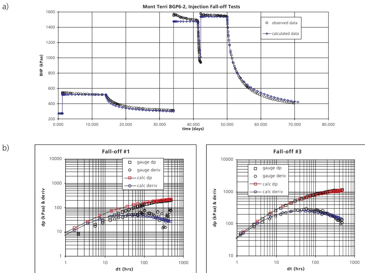
Figure 4.12: Hydro-mechanical modelling of the interference test in BGP-6 – simulated interval pressures. Note that only the fall-off events (HIS events) were fitted, whereas the HI events were given by prescribed pressure: (a) The overall fit of interval pressure and (b) the diagnostic plots of the fall-off events are satisfactory (after TN 2000-21).
