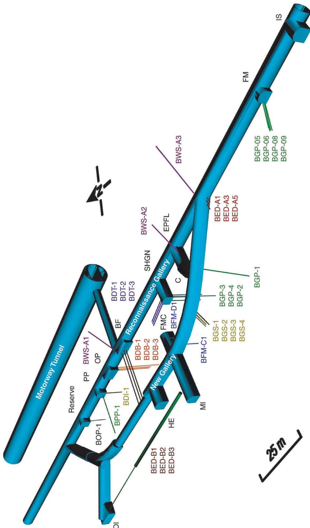
Figure 2.2: 3D view of the Mont Terri site showing niches and boreholes of relevance for the synthesis of hydrogeological investigations.
