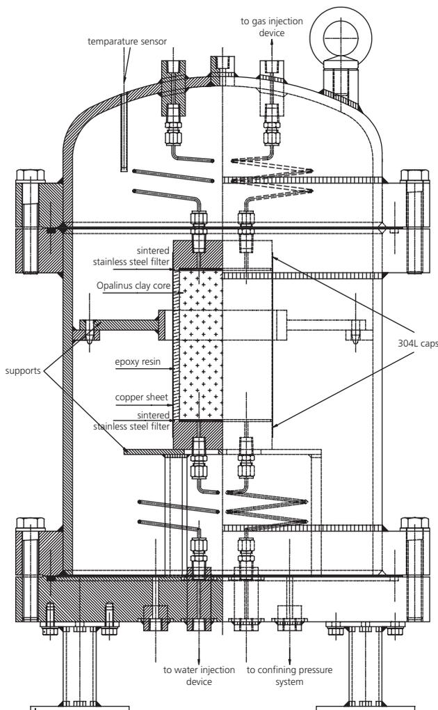
Figure 5.1: Schematic view of SCK-CEN's isostatic cell and sample assembly for the Opalinus Clay samples as part of the GP experiment (after TN 99-58).
