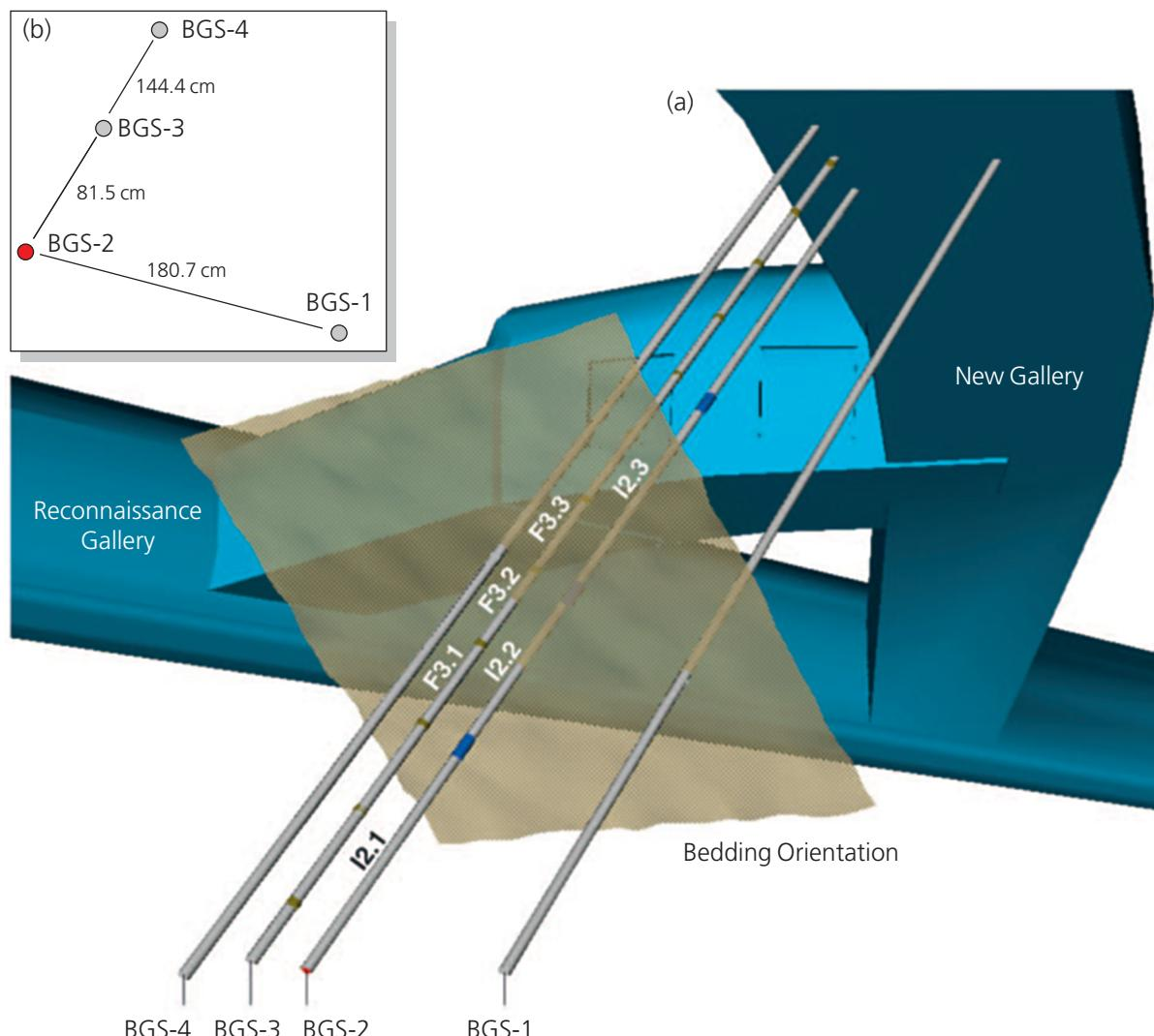
Figure 5.4: Long-term gas injection experiment in the GP-A/GS site. (a) The test configuration consisted of two boreholes: BGS-2 was equipped with a triple packer system, BGP-3 with fixed installed micrometers. (b) Shows a plan view drawn perpendicular to BGS-2 through the centre of test interval I2.2. (c) At gas injection pressures of more than 2 MPa, a significant mechanical response is observed in BGP-3 (after Enachescu et al. 2002). (c) on page 77.
