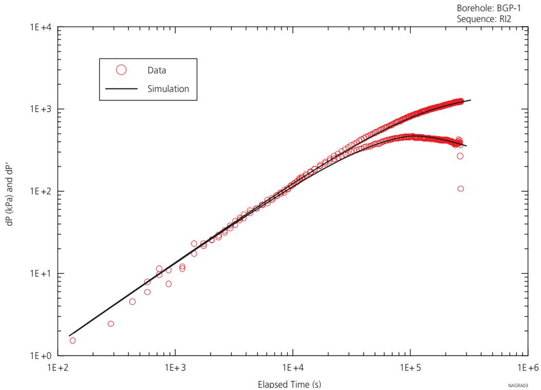
Figure 4.2: Baseline simulation of pressure change (dP) and log-derivative (tdP/dt) during BGP-1 – R12 constant-rate injection test (after TN98-24). The diagnostic log-log derivative plot allows for systematic flow model identification.
