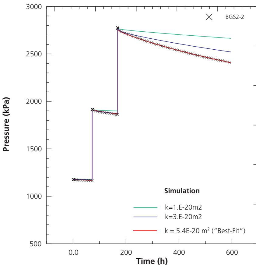
Figure 5.8: Modelling of the gas test sequence in BGS-2/12 with TOUGH2. The sensitivity of the pressure response to the variation of intrinsic permeability is shown. The third pressure step is most sensitive to permeability. The best-fit intrinsic permeability is 2 to 3 times higher than the best-fit permeability, determined from hydrotest analysis (after Senger et al. 2002).
