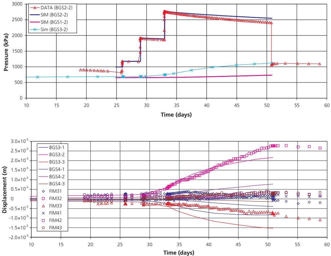
Figure 5.9: Coupled 3D hydro-mechanical simulation: Pressure history in BGS-2/1/2, BGS-1/1/2 and BGS-2/1/3, and FIM data in boreholes BGS-3 and BGS-4. Assumptions: Pressure-dependent permeability over the entire test interval, linear-elastic geomechanical model with an E modulus of 6 GPa (after Senger et al. 2002).
