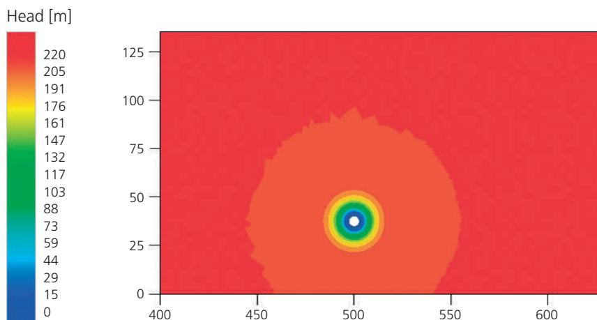
Figure 4.27: Simulation of the distribution of pressure head on a plane projected perpendicularly through the reconnaissance gallery and the new gallery at approximately tunnel meter RG 970. Hypothetical points in time: (a) end of April 1998, (b) end of July 2000.
