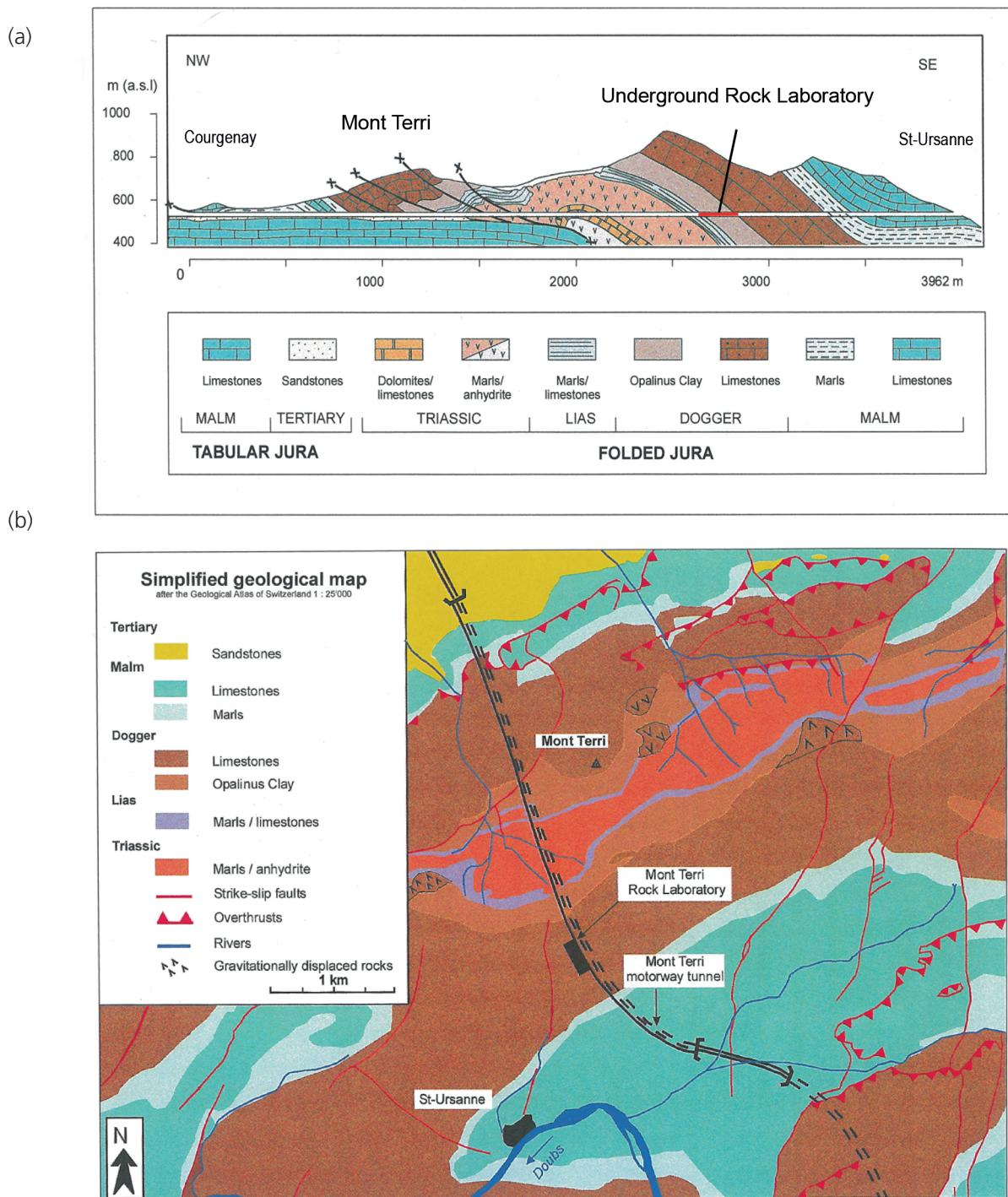
Figure 4.14: (a) Simplified geological cross-section through the Mont Terri anticline along the motorway tunnel, showing the location of the Mont Terri rock laboratory (Thury & Bossart 1999) and (b) simplified map of the Mont Terri anticline.
