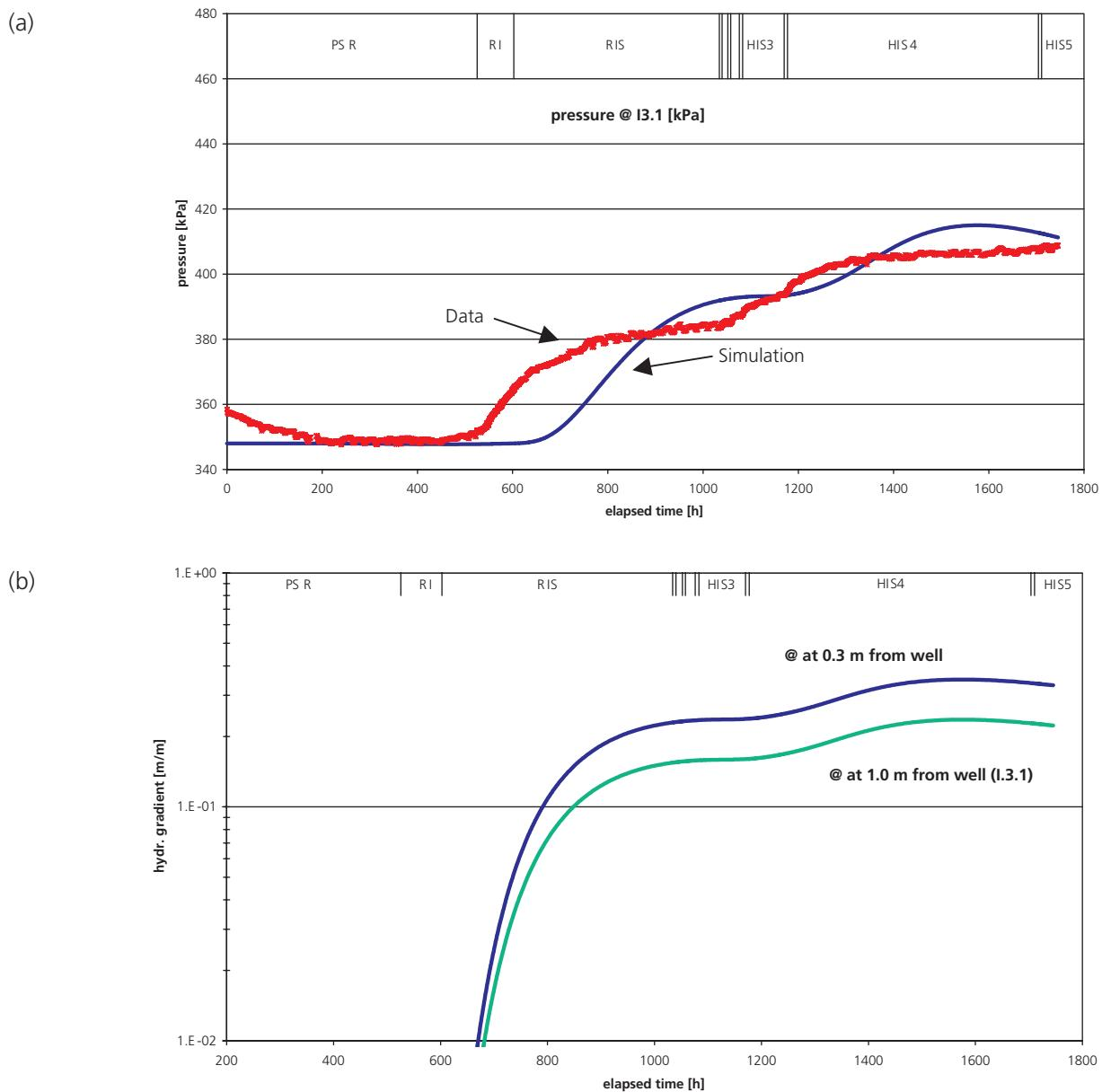
Figure 4.7: Simulation of the crosshole response in BGP-3/I1 to a sequence of rate injection and head injection tests in BGP-4 (TN 98-24): (a) a satisfactory fit of the response in BGP-3 by inverse modelling was not achieved; (b) hydraulic gradient at a distance of 0.3 m and at the location of borehole BGP-3/I1. The gradients are computed based on a radial flow model.
