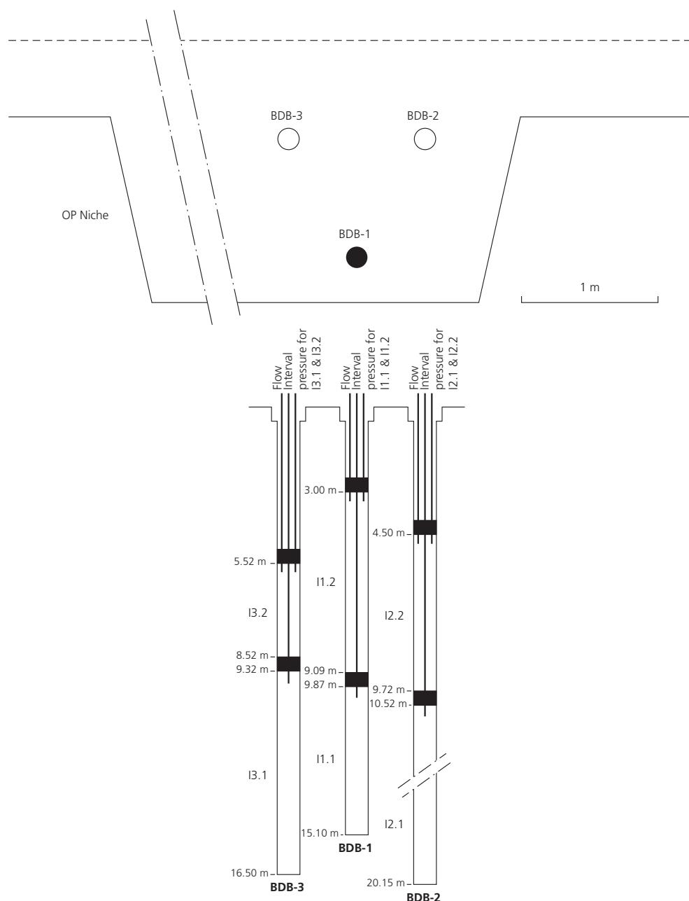
Figure 3.4: Map view and cross-section of the set-up for the systematic investigation of the impact of the drilling technique and the chemical composition of the test fluids on packer test results. The three boreholes BDB-1, BDB-2 and BDB-3 were drilled with air, silicate/polymer mud and potassium-chloride/polymer mud, respectively. Synthetic porewater was used for hydraulic testing.
