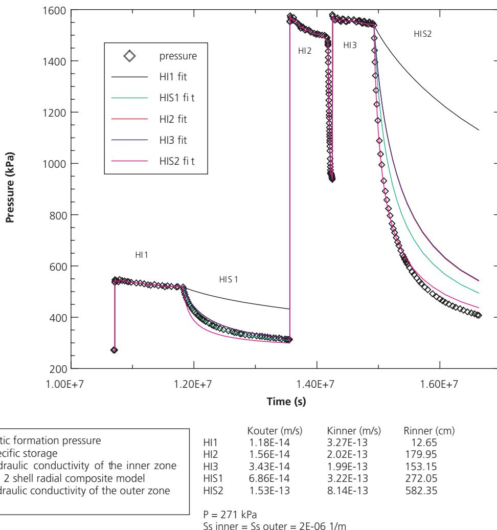
Figure 4.11: Inverse modelling of the packer test conducted in BGP-6 using a finite skin model (inner zone / outer zone) exhibits difficulties in simulating jointly the HI1 / HIS1 sequence and the HI2&3 / HIS2&3 sequence. The analysis of HI1 / HIS1 gives a hydraulic conductivity in the order of 1 to 3 E-14 m/s. The two latter test sequences suggest values in the range 7E-14 and 2E-13 m/s (after TN 2000-21).
