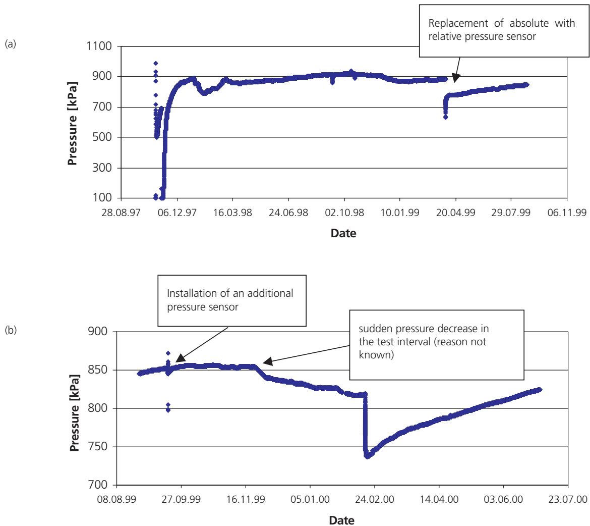
Figure 4.8: Pressures recorded in borehole BOP-1, (a) prior to fluid exchange, and (b) shortly before and after the fluid exchange with de-ionised water on February 16<sup>th</sup>, 2000.
