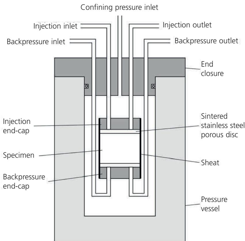
Figure 3.2: Schematic of the pressure vessel and specimen assembly for the laboratory pilot study.
