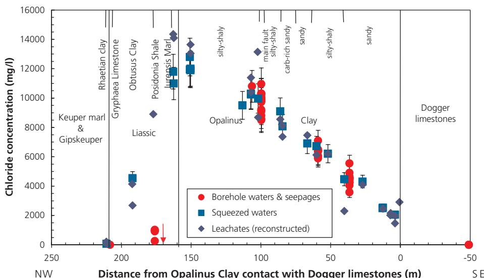
Figure 4.15: Chloride profiles as an indirect evidence for groundwater flow conditions in the Opalinus Clay and in the adjacent stratigraphic formations. The chloride profile shows a gradual decrease in concentrations towards the Lower Dogger, which is an indication for more intense groundwater flow in this formation (after Pearson et al. 2003).
