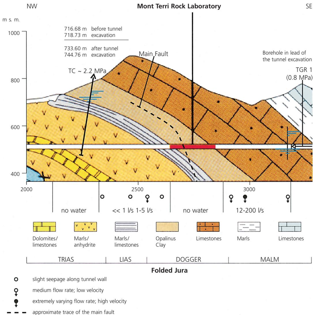
Figure 4.21: Cross-section through the Mont Terri site with piezometric levels (TN 99-22).
