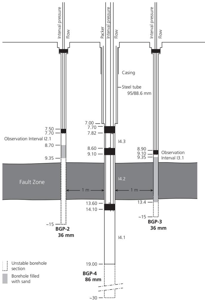
Figure 3.1: Piezometer systems tested in Phases 1 to 4 of the Mont Terri research program: (a) classical inflatable triple packer system in borehole BGP-4 and mechanical minipacker systems in BGP-2 and BGP-3 as applied in the GP experiment / Phase 2 (TN 96-27) and (b) PP system developed in the PP experiment / Phases 1 and 2 (TN 97-01 & TN 97-02).
