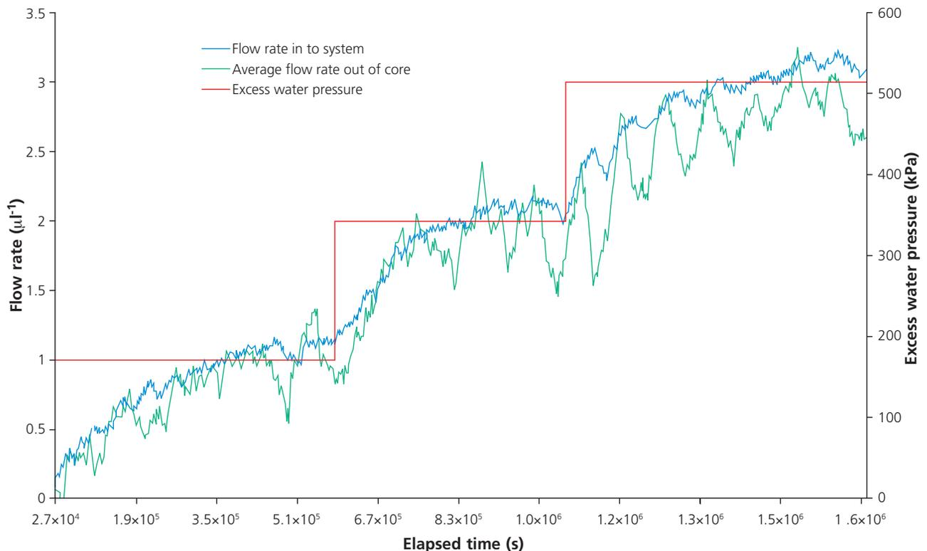
Figure 4.5: Permeameter test conducted in the OP experiment (TN 97-39). Linearity between flow and pressure is proven for hydraulic gradients  $> 1000 \text{ m/m}$  (Figure taken from TN 97-26).
