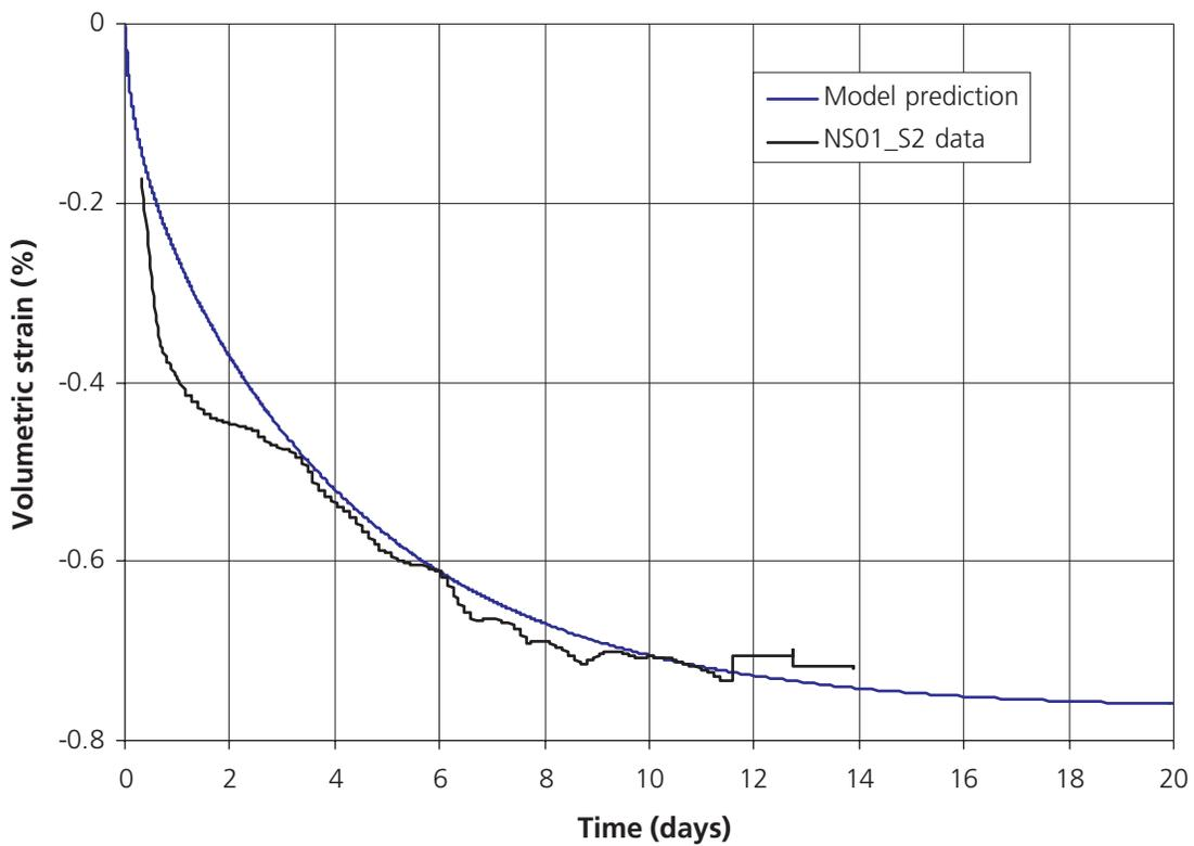
Figure 5.2: Model predictions of flows and volumetric strain as a function of time using equations (25) and (26) compared to the data from laboratory pilot study NS01 Stage 2. Negative volumetric strain indicates swelling of the sample.
