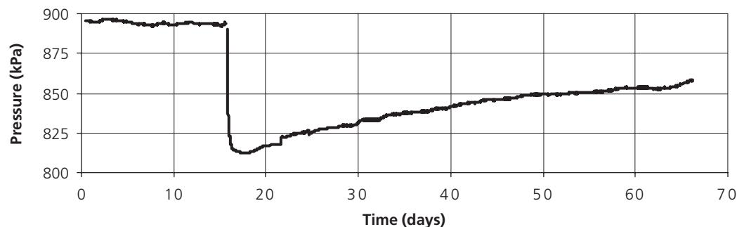
Figure 4.2: The pressure evolution for Phase 2, replacement of the test section fluid with de-ionised water. The data have been plotted starting from 1 February 2000.
