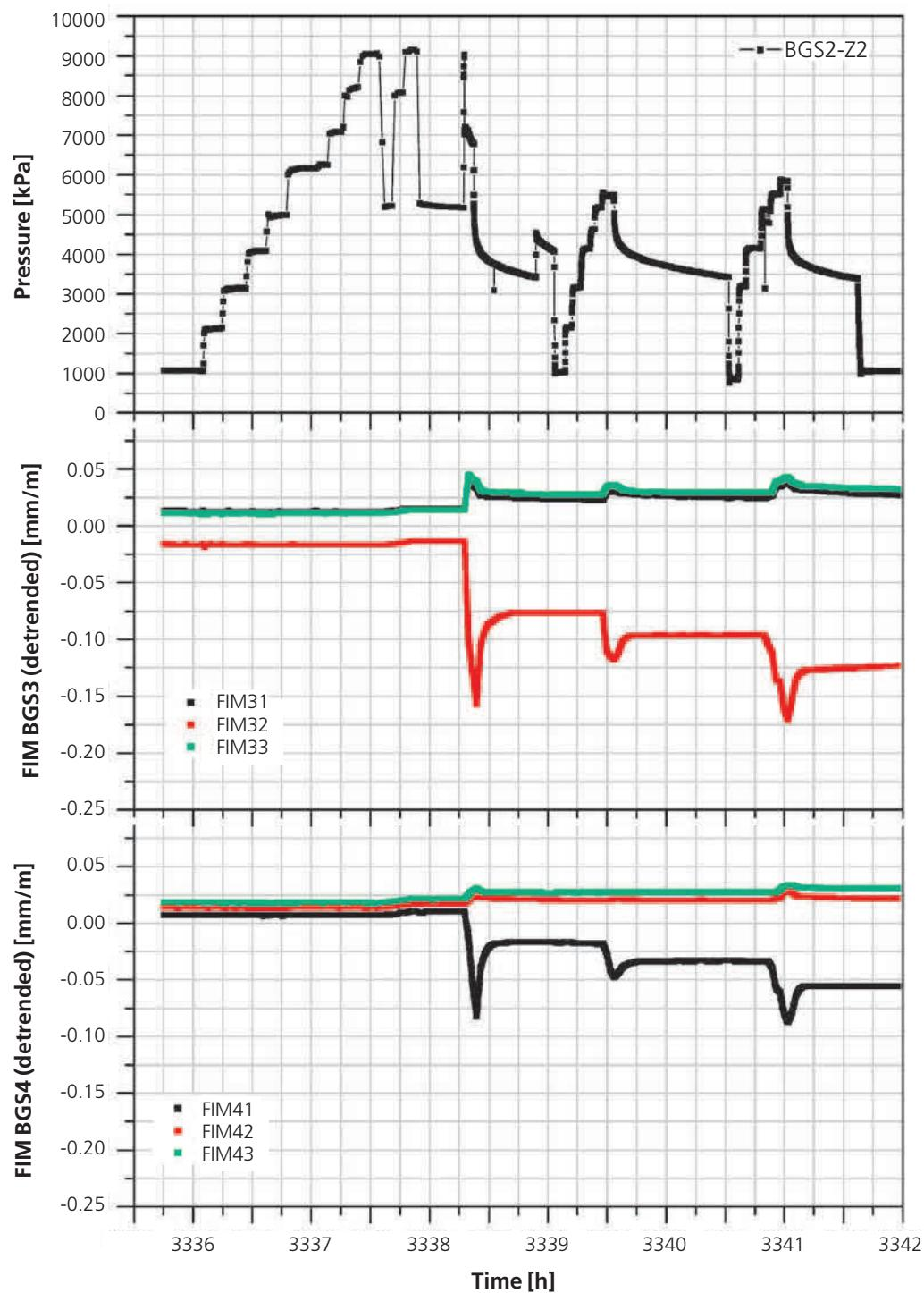
Figure 5.5: Sequence of hydrofrac and re-fracture events in test interval I2.2 of borehole BGS-2. Pressure transients in interval I2.2 of borehole BGS-2 and displacements measured in BGS-3 and BGS-4 (after Enachescu et al. 2002).
