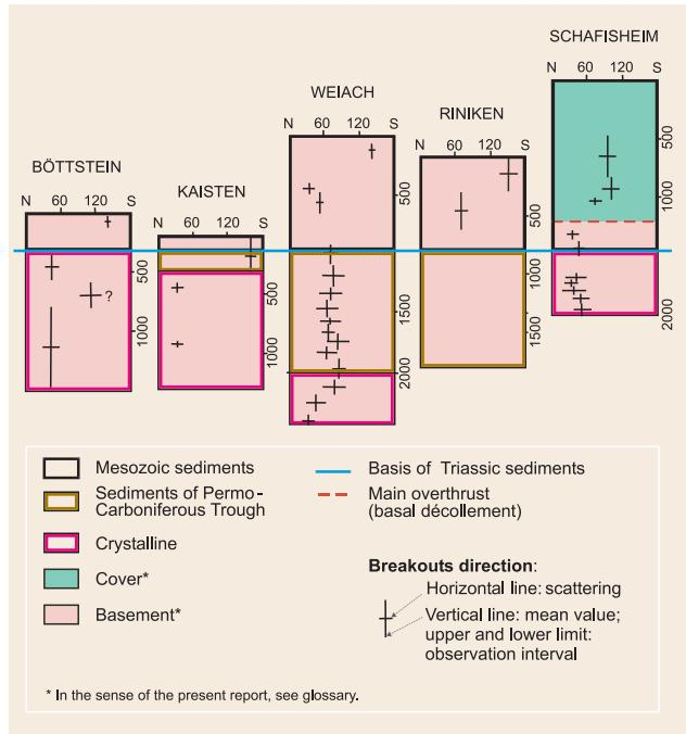
Figure 2: Average direction values of breakouts measured in five deep boreholes in the northern Jura Mountains and foreland, after MÜLLER et al. (1987), modified. Directions in [°].
