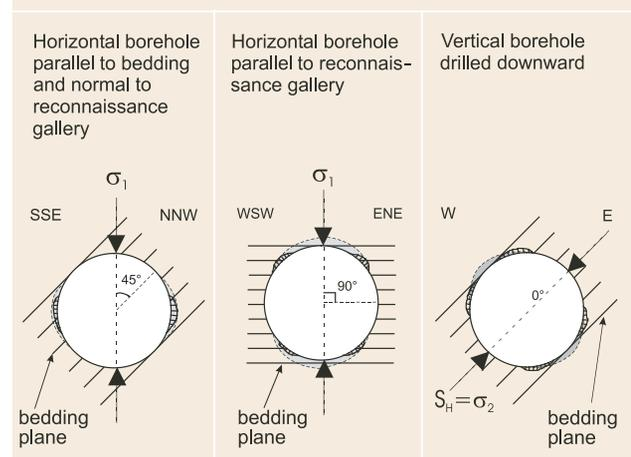
Figure 9: Expected stress-induced breakouts observed in the Opalinus Clay of the Mont Terri Rock Laboratory for three different borehole directions. Hatched zones represent stress-induced breakouts expected in anisotropic rocks. The grey zones represent stress-induced breakouts expected both in isotropic and anisotropic rocks.
