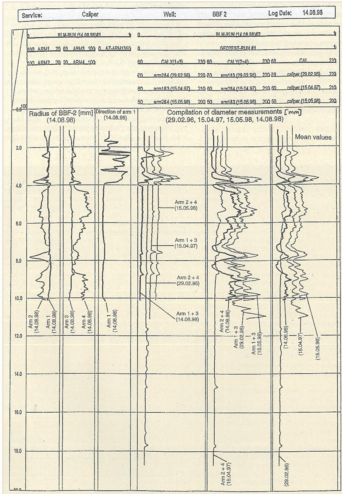
Figure 11: Caliper logs in the fluid-filled borehole BBF-2, niche BF – facsimile of field record (for location see Figure 3).
