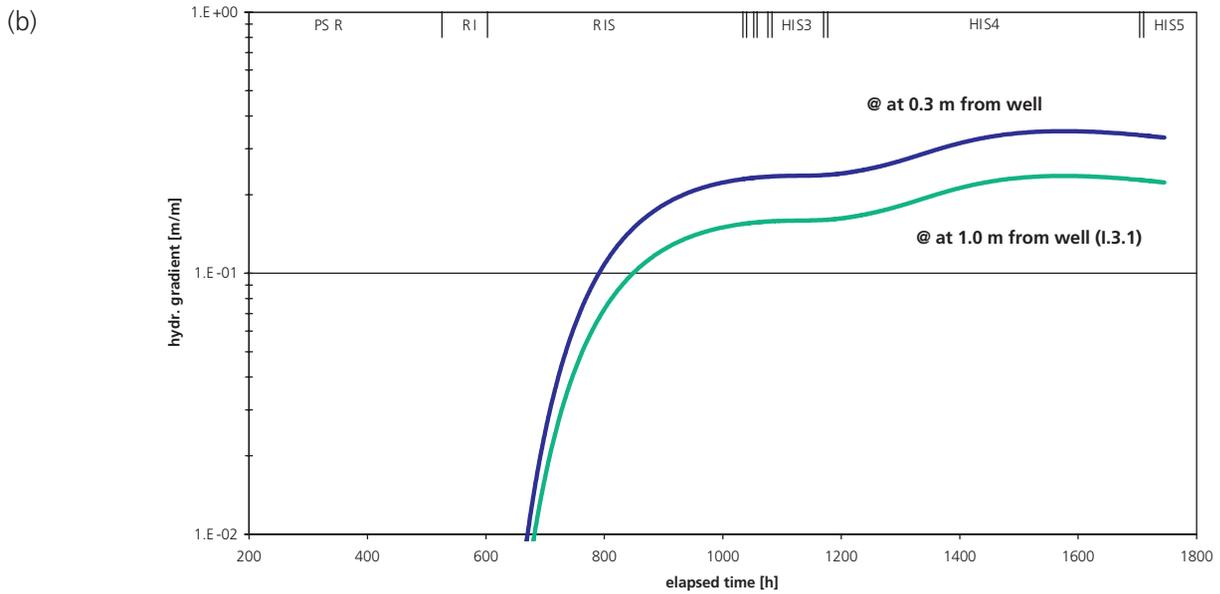
Figure 4.7: Simulation of the crosshole response in BGP-3/1 to a sequence of rate injection and head injection tests in BGP-4 (TN 98-24): (a) a satisfactory fit of the response in BGP-3 by inverse modelling was not achieved; (b) hydraulic gradient at a distance of 0.3 m and at the location of borehole BGP-3/1. The gradients are computed based on a radial flow model.
