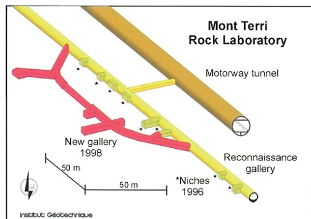
Figure 2.1: (left) View toward the North, with St-Ursanne in the foreground and Mont Terri in the center with the red arrow indicating the southern entrance of the motorway tunnel. (right) 3D view of the Mont Terri Rock laboratory.
