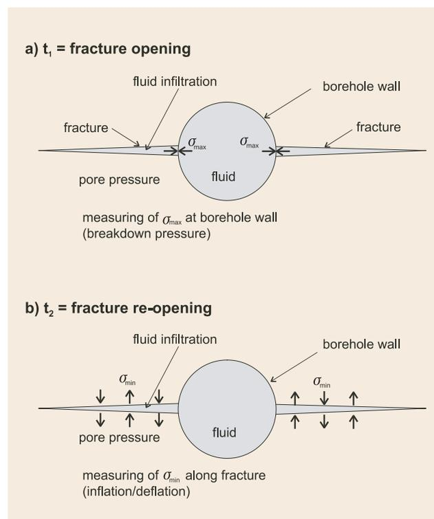
Figure 5: Hydraulic fracturing method: a) first fracture opening and b) fracture re-opening.
