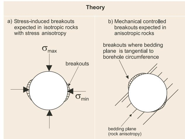
Figure 6: Borehole breakouts due to a) stress redistribution around borehole in isotropic rocks and b) anisotropic rock fabric such as the pronounced bedding planes.
