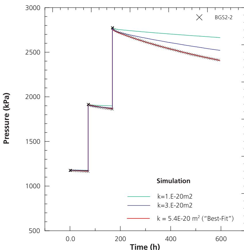
Figure 5.8: Modelling of the gas test sequence in BGS-2/I2 with TOUGH2. The sensitivity of the pressure response to the variation of intrinsic permeability is shown. The third pressure step is most sensitive to permeability. The best-fit intrinsic permeability is 2 to 3 times higher than the best-fit permeability, determined from hydrotest analysis (after Senger et al. 2002).
