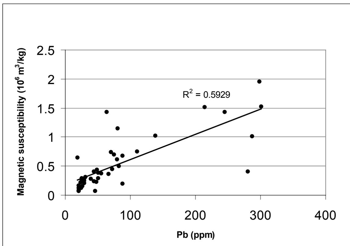
Figure 2. Basel region: topsoil magnetic susceptibility versus lead content.
