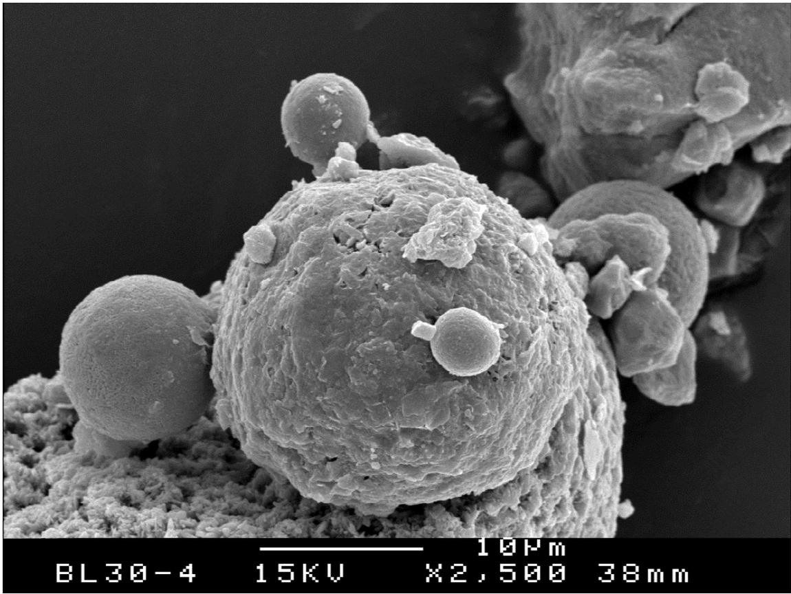
Figure 14. Scanning electron microscope image of magnetic extract from sample BL 30 Basel country
