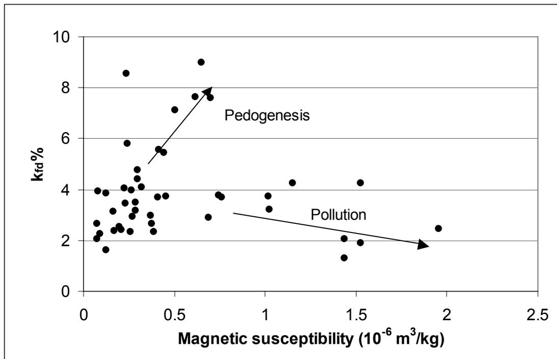
Figure 7. Basel region: Topsoil frequency dependent susceptibility versus magnetic susceptibility.
