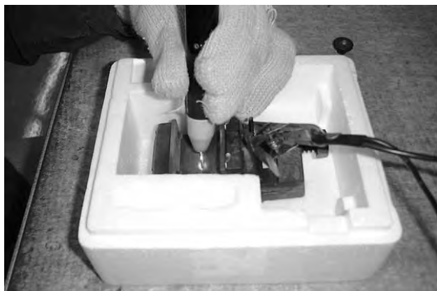
Figure 3.4.3: Picture at the top shows the steps described in the text of the capsule preparation from a cut gold tube (left) to the capsule after the experiment (right). The lower picture shows the plasma-arc welding with the sample in liquid nitrogen (−196 °C).
