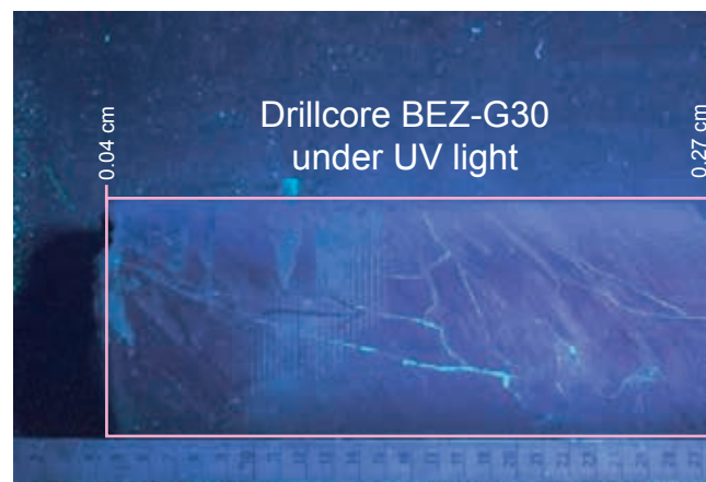
Mapping of impregnated fractures with epoxy resin
